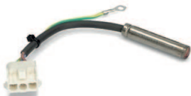
RG0V1786 Resistenza cartuccia 25W 230V, Ø10 x 51,00mm Cartridge heating element 25W Ø10 x 51,00mm
